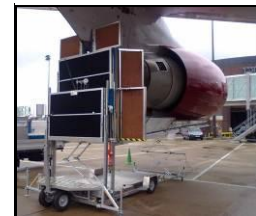
G4C lifted under Engine
